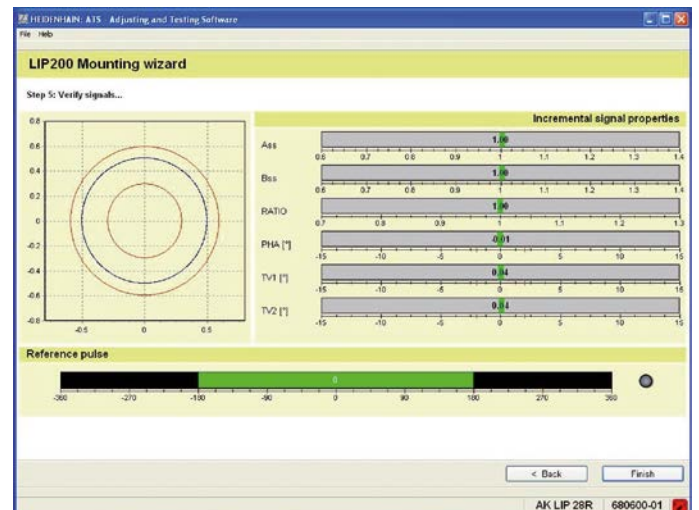
Commissioning using PWM 20 and ATS software
