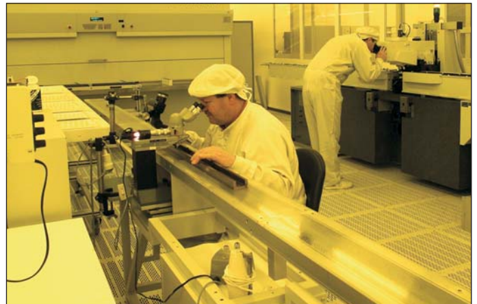
Linear scale inspection station in the lithography area
