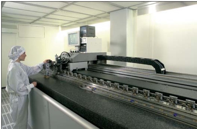
Measuring machine for linear scales
